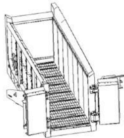
Goose neck and doors swing open for complete combustion chamber access
